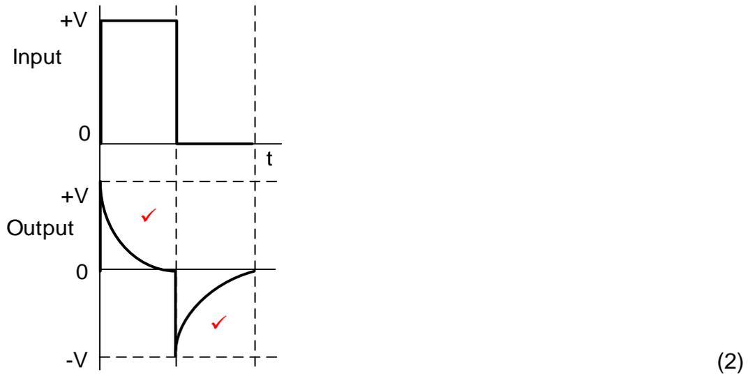
5.7.2 When a square wave is applied to the input, both plates of the capacitor immediately charges up to the potential of the input. ✓ The left hand plate of the capacitor is kept at that potential for as long as the square wave is high. ✓ The right hand plate of the capacitor will discharge through the resistor to 0 V ✓ at a rate determined by the RC time constant of the circuit. (3)
