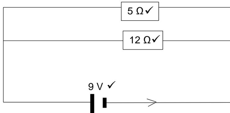
**NOTE/NOTA:** Penalise once if the resistors and the cell are not connected in parallel
